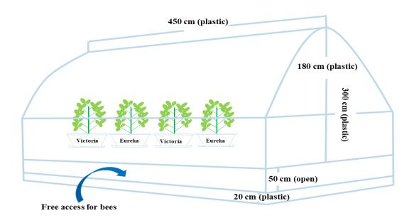
FIGURE S1 | Diagram of the plastic greenhouse.
