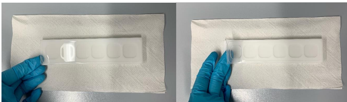
Supplementary Figure 8: Cautiously elevate the thin layer of polymerized PDMS surrounding the entities (a) before carefully detaching the PDMS from the mold (b).
