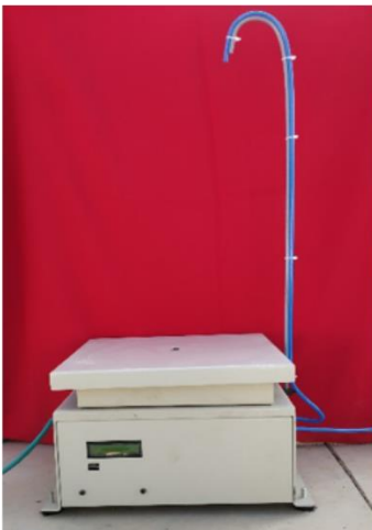
Figure S1: Minilysimeter (MLM) based drought-simulator platform for stress imposition protocol in rice. (A) Experiment 1 with 10 L capacity pots for protocol standardization during the seedling stage and (B) pots of 20 L capacity for inducing gradual stress in 17 genotypes were placed on lysimeters with the automated irrigation facility. (C) Load cell balance platform along with an irrigation pipe. (D) Overall view of the drought-simulator phenomics facility at University of Agricultural Sciences, Bangalore, India.
