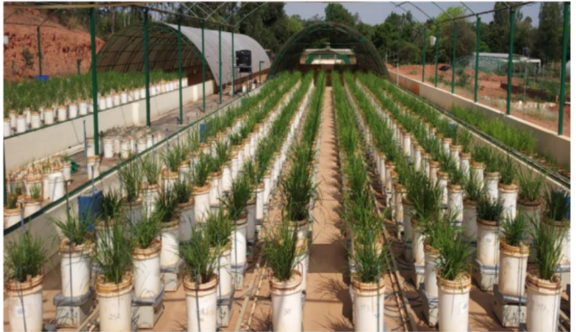
Figure S1: Minilysimeter (MLM) based drought-simulator platform for stress imposition protocol in rice. (A) Experiment 1 with 10 L capacity pots for protocol standardization during the seedling stage and (B) pots of 20 L capacity for inducing gradual stress in 17 genotypes were placed on lysimeters with the automated irrigation facility. (C) Load cell balance platform along with an irrigation pipe. (D) Overall view of the drought-simulator phenomics facility at University of Agricultural Sciences, Bangalore, India.
