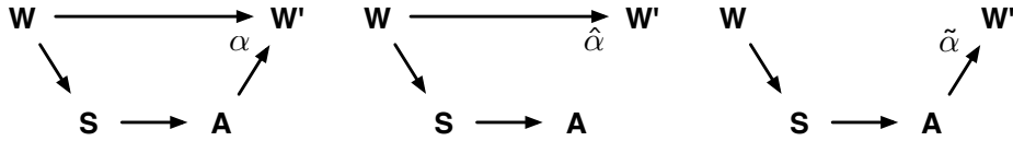
Figure 8: Visualisation of the two concepts MC_A and MC_W . Left-hand side: causal diagram for a reactive system. Centre: causal diagram assuming no effect of the action A on the next world state W' . Right-hand side: causal diagram assuming no effect of the previous world state W on the next world state W' .
