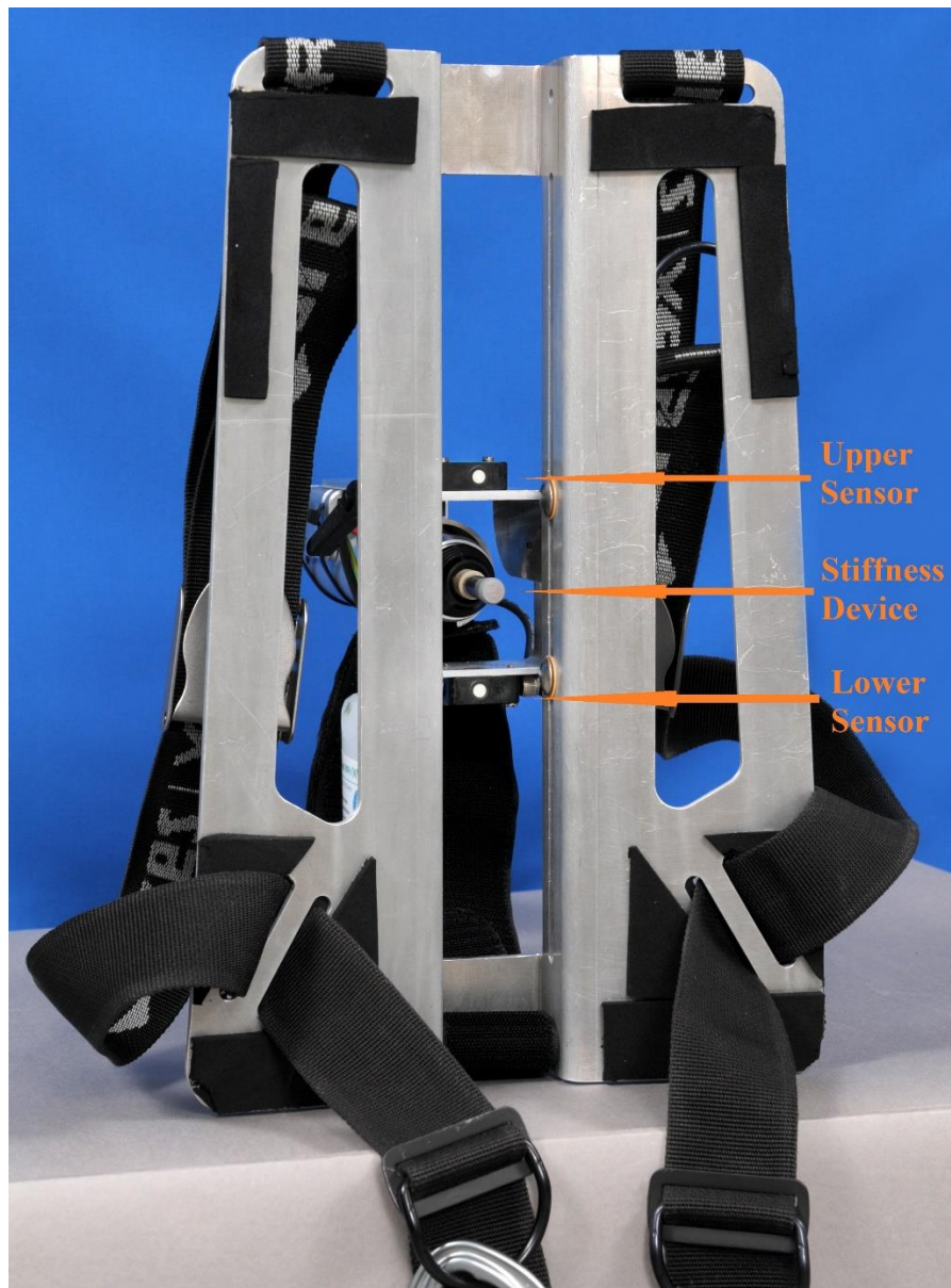
Figure S1 The measurement setup with stiffness device (SD) and the two ultrasonic distance sensors
