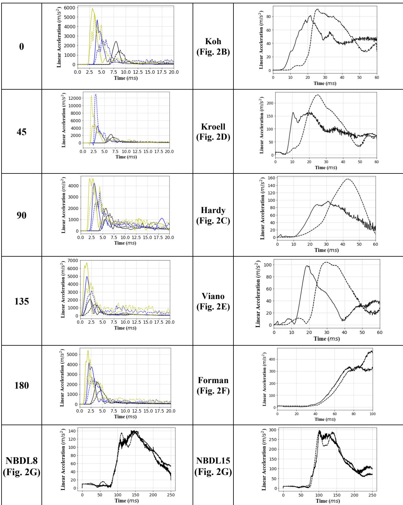
1 **Figure A1:** Linear Acceleration of Head CG. M50-O (dashed), M50-OS (solid) at 3 (blk), 6
