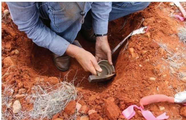
Collecting samples along the soil profile
