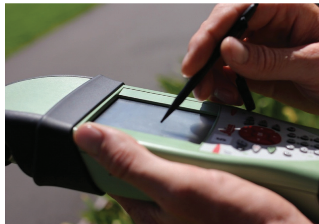
The differential GPS (DGPS) unit used in the AusPlots Rangelands survey protocols
