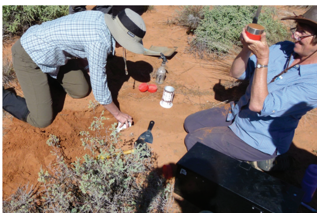
Collecting Soil Bulk Density samples using the AusPlots Rangelands Survey Protocol
