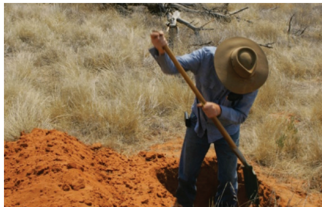
Digging a pit to expose the soil profile
