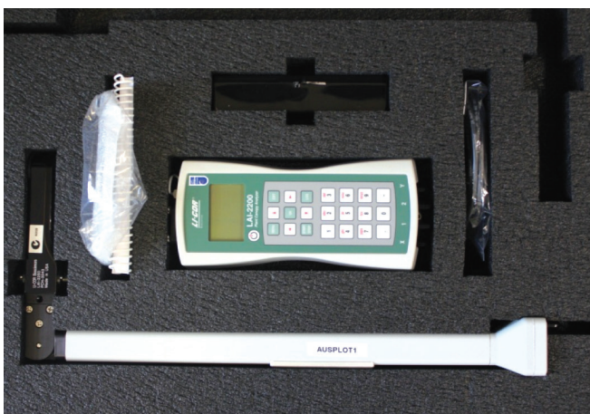
The LAI-2200 used in the AusPlots Rangelands Survey Protocols
