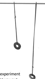
Think up two experiments to check if the length of the rope affects the period. For each experiment you have to choose the length of the rope, how far you pull it aside and how much weight you put on the pendulum
