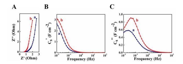
Figure S1. (A) Nyquist plot of complex impedance and (B,C) frequency dependence of complex capacitances (B) Cs' and (C) Cs" for (a)ZnFe-CNT and (b) ZnFeCB-CNT.
