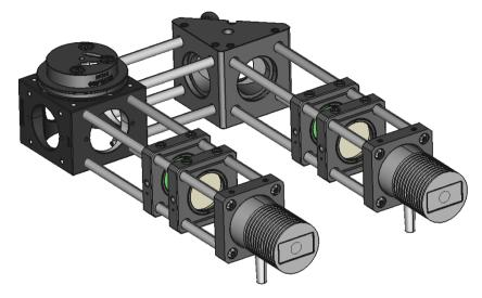
10. Fix the dichroic mirror mount containing filter MD498 - GFP to the system
