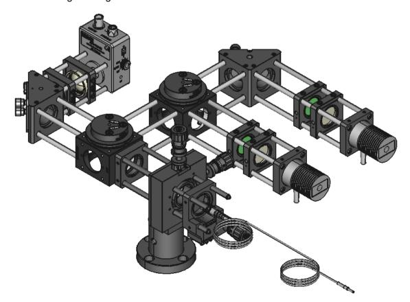
20. Mount lens tubes (SM1L03, Thorlabs) to shield background light from the emission pathway.
