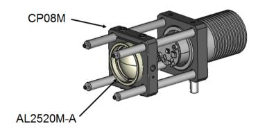
4. Mount the bandpass filters in the LED beam path
