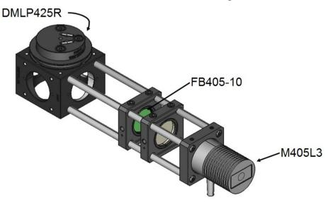
9. Fix the two mirror mounts together and co-align the beams using adjustment screws.
