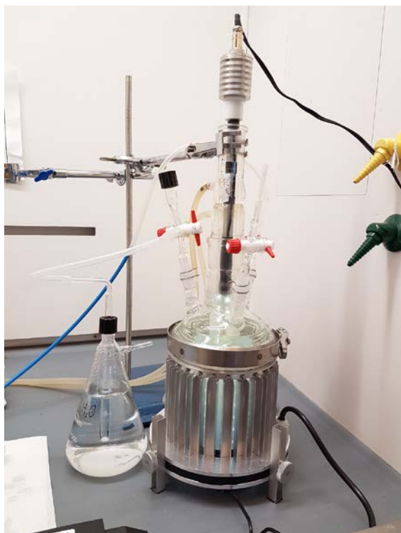
Supplementary Figure 1. Picture of the reaction system used for the photocatalytic runs.
