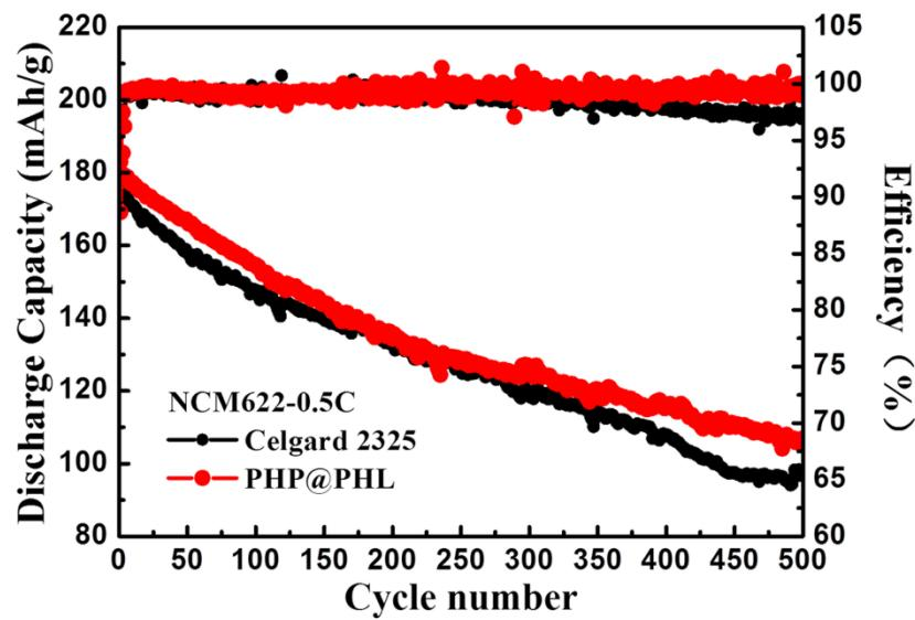
Figure S5. Cycling performance of the NCM622/Li cells with Celgard 2325 and PHP@PHL membrane at 0.5C.
