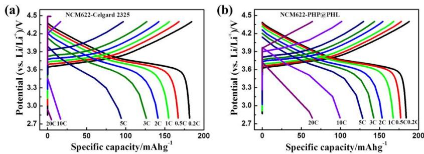
Figure S6. Charge-discharge voltage profiles of the NCM622/Li half-cells with (a) Celgard 2325 and (b) PHP@PHL membrane at different C rates.
