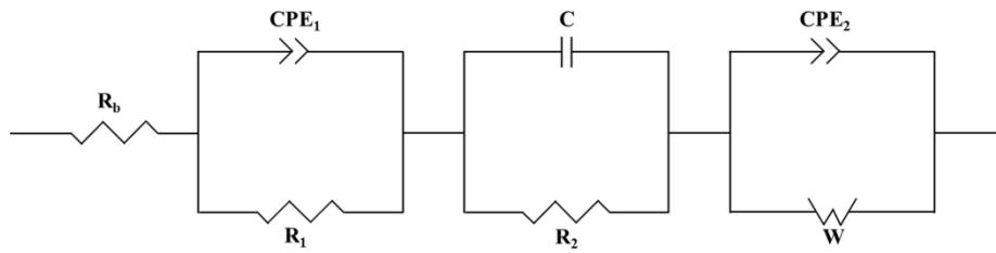
Figure S4. Equivalent circuit of the electrochemical impedance spectroscopy results in figure 6 (Li et al., 2013).
