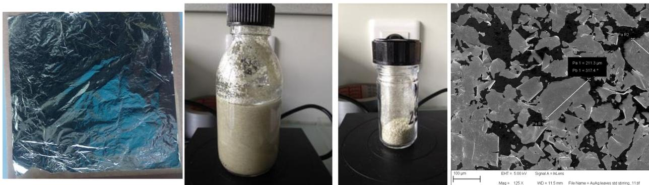
*Figure B : Photos, from the left: a white gold leaf (Au<sub>35</sub>Ag<sub>65</sub>); fragmentation under magnetic stirring in UP water; powder eventually obtained (after 8 h). SEM image: Au<sub>35</sub>Ag<sub>65</sub> fragments.*
