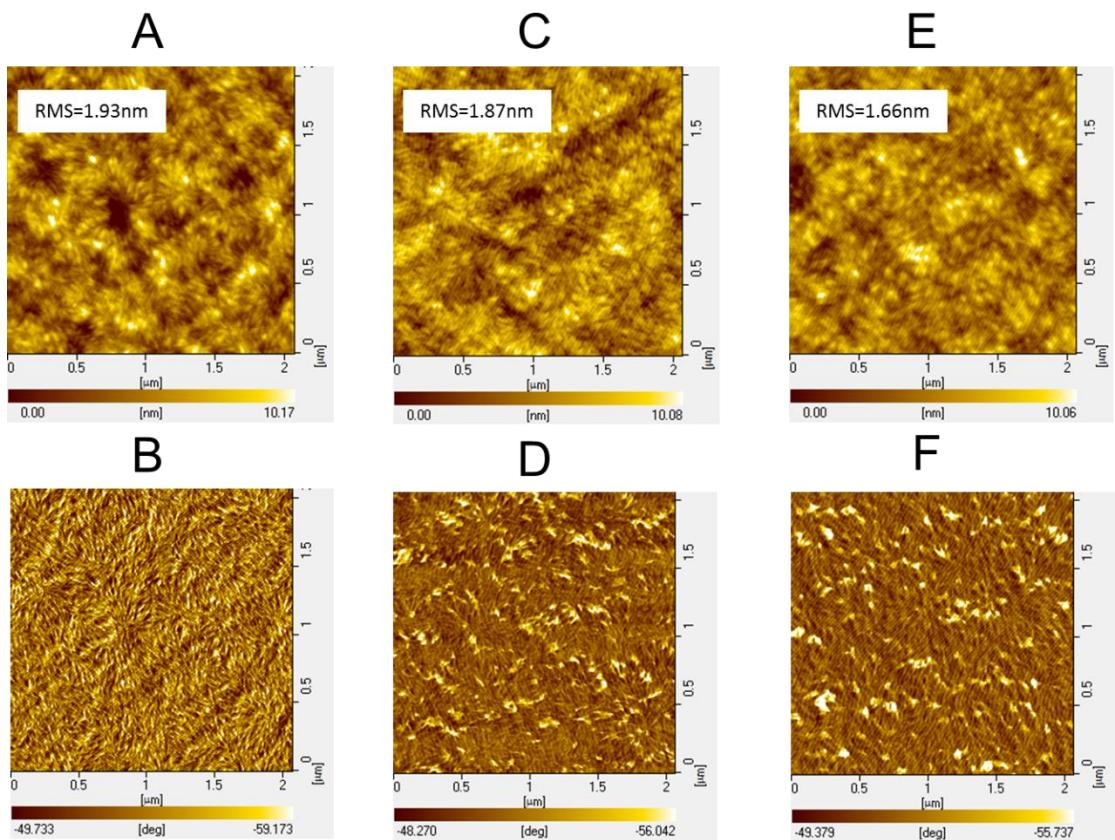
**Figure S2.** Height images (A, C, E) and phase images (B, D, F) of PBDB-T:ITIC (1:1), PBDB-T:ITIC:PC<sub>71</sub>BM (1:0.8:0.2) and PBDB-T:PC<sub>71</sub>BM (1:1) blend films, respectively.
